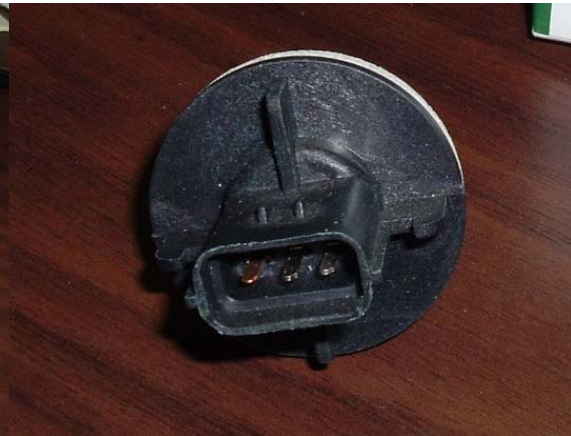
The new bulb holder has three terminals. One for ground, one for parking lights, and the other for turn signal.
