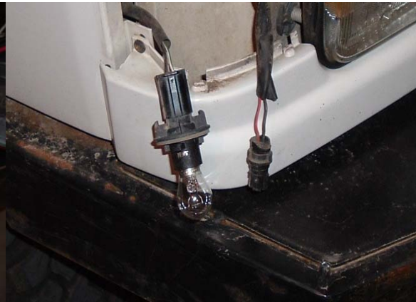
The new bulb holder has three terminals. One for ground, one for parking lights, and the other for turn signal.
