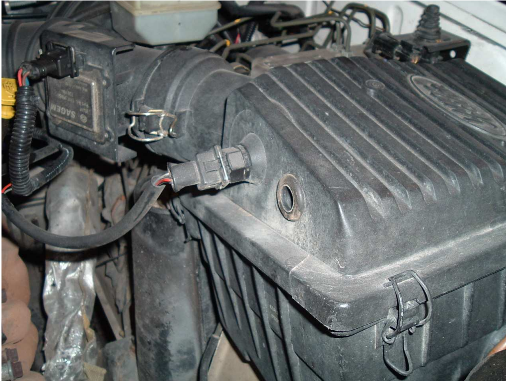
Airbox with grommet installed
